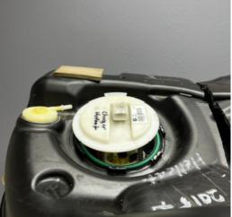
11. Next, slowly remove the top hat, this will separate from the main body of the pump. The feedline and siphon return line should now be visible, disconnect these from the body of the pump.
