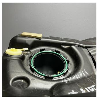
14. Be sure to cover the opening into the tank to ensure no trash enters the fuel system.
