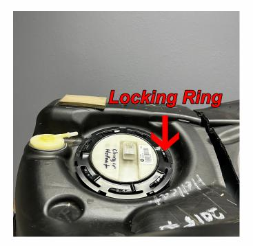
10. The OEM Dodge pump assembly is spring-loaded and will pop up as soon as the lock ring is released.
