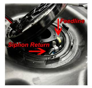
24. With the body properly connected reinstall the top hat bolts and tighten in a cross pattern(58 in/lbs) insuring proper seating of the O-ring.
